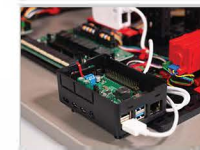
Raspberry Pi (IoT Gateway)
