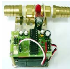
Demo 9 Water Valve Control
